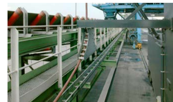
A cable guide alongside the conveyor belt also saves space.
