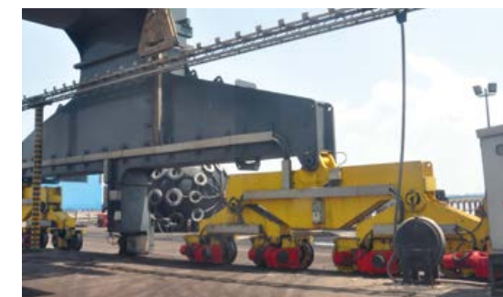
High-level cable guide arrangement allows vehicles to travel under the supply cable.
