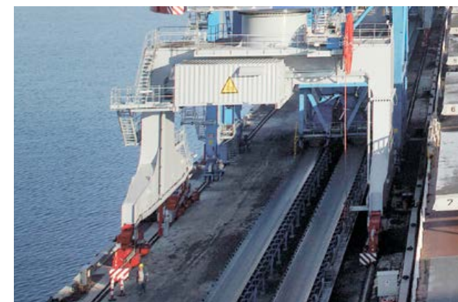
Conveyor belts running under the portal.
