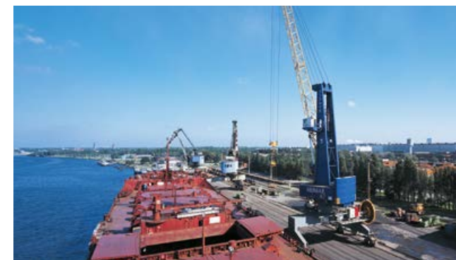
High-performance Konecranes Gottwald Portal Harbor Cranes use the rails on existing quays.
